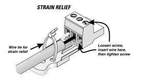
For heavy-duty input cables, the use of connectors with integral strain relief is recommended. These connectors have a large plastic tab molded as part of the assembly which provides an area to tape or tie-wrap the cable to. At the time of this writing, only the 3-pin with the strain relief was available through QSC . See Section 6 (Appendix) for connector part numbers.
